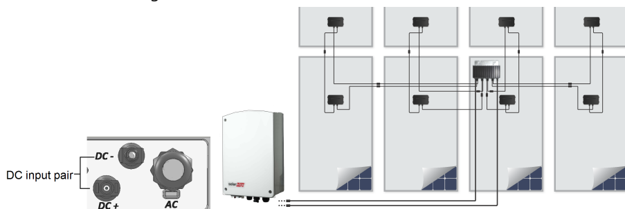
Figure 14: Inverter DC Connections
